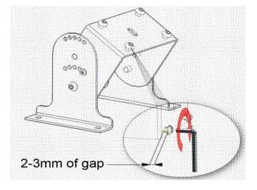
**Step 4:** Put the heater on the wall, slide it into bracket part 1 ①.
