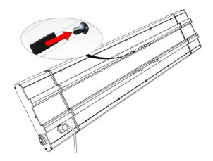
Step 2: Install the bracket on the back of the heater.
