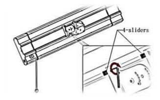
Step 3: Fix bracket part 1 (1) on the wall, tighten the four nuts (a part
