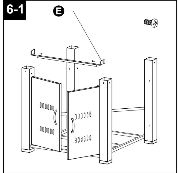
6-2. Do not put door bracket too close to the doors to ensure two doors can open easily.
