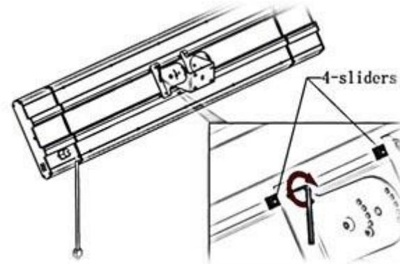
**Step 3:** Fix bracket part 1 ① on the wall, tighten the four nuts (a part of anchor bolt M6\*50) ② with M6 spanner ⑨
