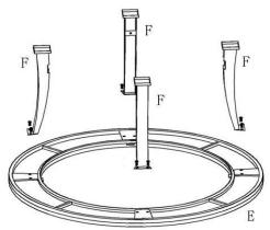
Step 3: Attach Support Ring (G) to 4 Legs (F) by using 4pcs M6\*12 bolts(AA) tightened, once ring is attached tighten all the bolts.
