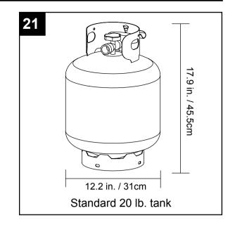
any other enclosed area. The maximum inlet gas supply pressure: 250 psi /1750 kPa.
