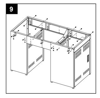
10-1. Use 3 M6X12 Bolts to make the small bracket and back panel of the big box stable. 10-2. Use 2 M6X12 Bolts and 2 Flange Nuts to make the small bracket and side panels of the big box stable ( Nut inside, Bolt outside ).
