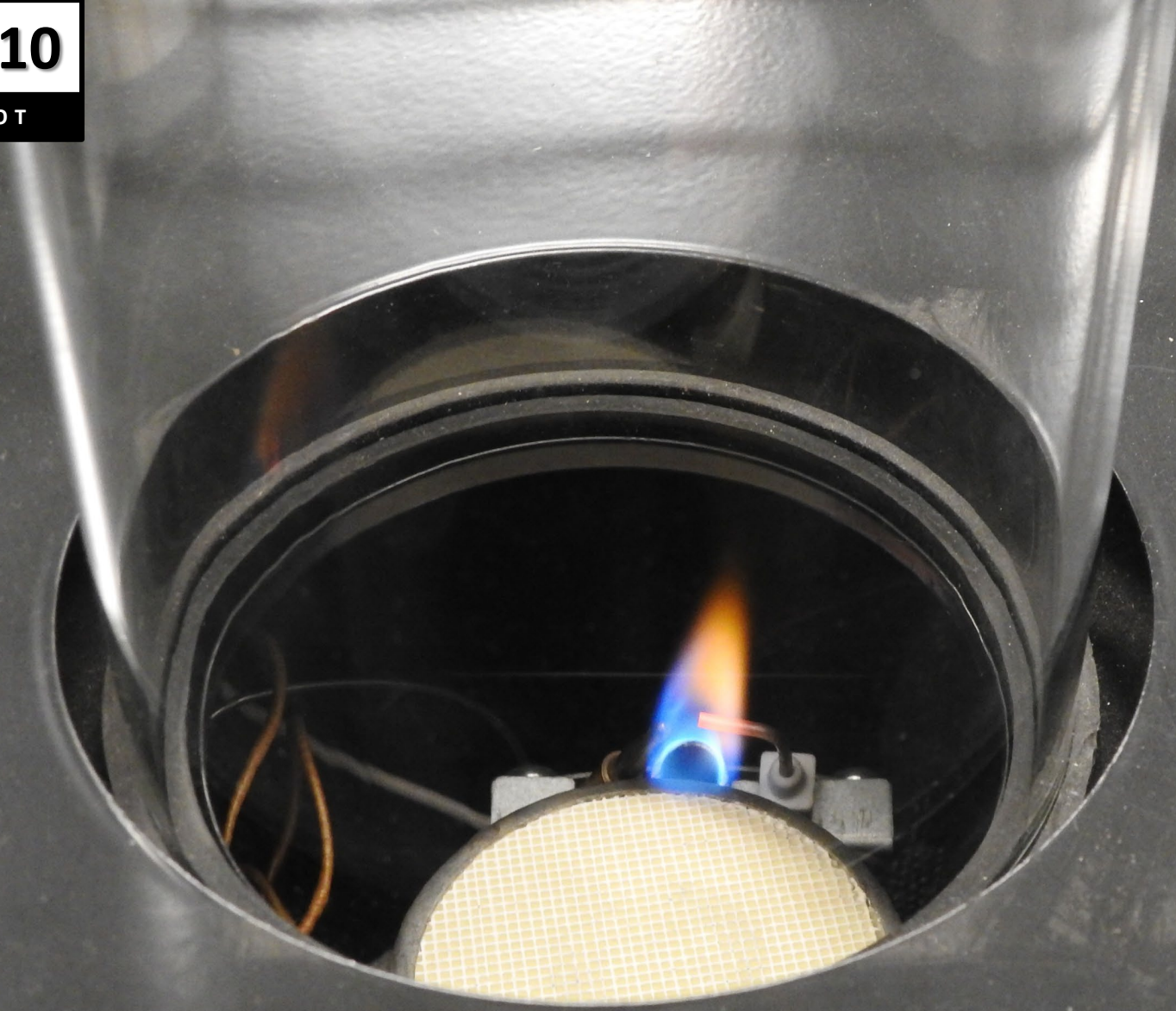
The pilot should be a nice blue flame as shown
