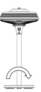
3. Put the power cord into the groove at the bottom of the base and then use 6x14 Phillips screws to lock it.
