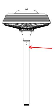
2. Put the power cord through the center hole of the base, and then screw the heater assembly clockwise into the base.
