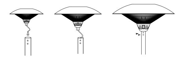
Step 4: Fix the Power cable on the Iron Base by using provided 6\*14mm (2) screws.
