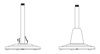
Step 2: Connect the middle tube with bottom tube by screwing them together. Connect the top tube with middle tube by screwing them together.
