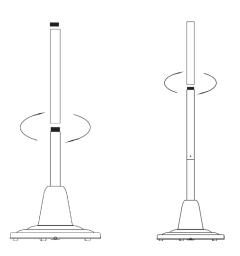
Step 3: **This step may require 2 people.** Feed the Power cable through the tubes and pull through the bottom of the base. Push the Heater Head onto the Top Tube and fix it in position using the provided 4\*10mm (2) screws.
